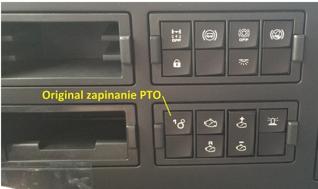
Picture 1 – Original switching on the PTO
