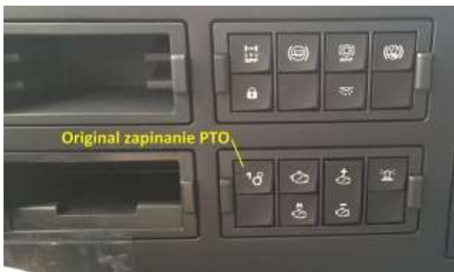
Picture 1 – Original switching on the PTO
