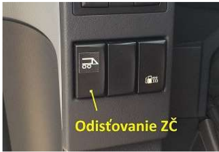
Picture 2 - releasing of the tailgate
